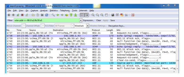
The packets containing data exchanged between the AP and the Iphone can now be interpreted by Wireshark.
