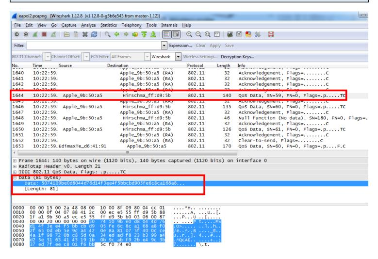
In the capture, the traffic between the iphone and the Access Point can be identified, but canno't be interpreted.
